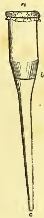
Pipette, serving as the stopper to the bottle. a , vulcanised india rubber, by pressing which fluid may be expelled from the tube. b , ground to fit the neck of the bottle. c , the orifice. § 139.
